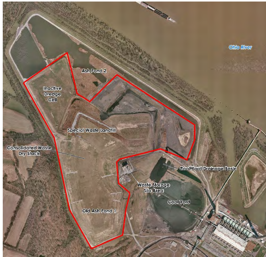
Figure 2: Consolidated Waste Dry Stack Unit Configuration
