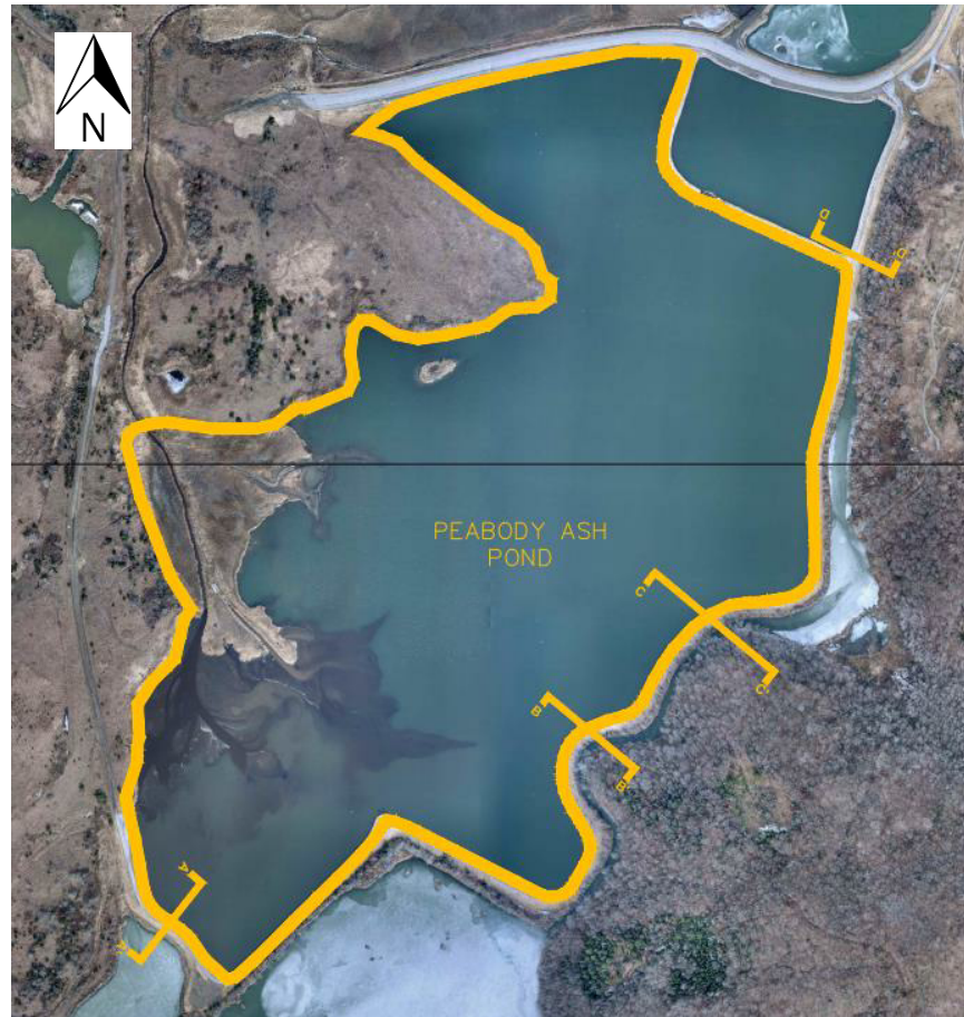
Figure 3. Peabody Ash Pond Critical Cross-Sections
