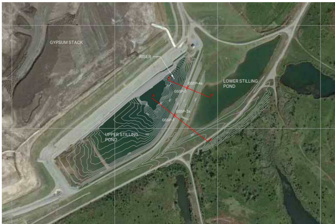
Figure 4. Gypsum Disposal Area Critical Cross-Sections
