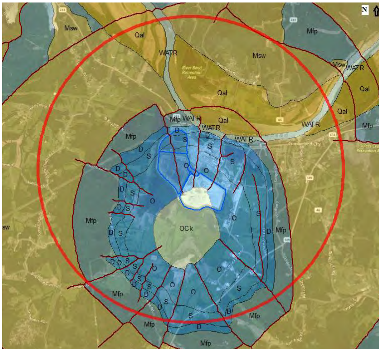
Figure 1. TVA Cumberland Fossil Plant study area (red); Geology and inferred faults (purple) from USGS Mineral Resources On-Line Spatial Data. Image source: Bing Maps.
