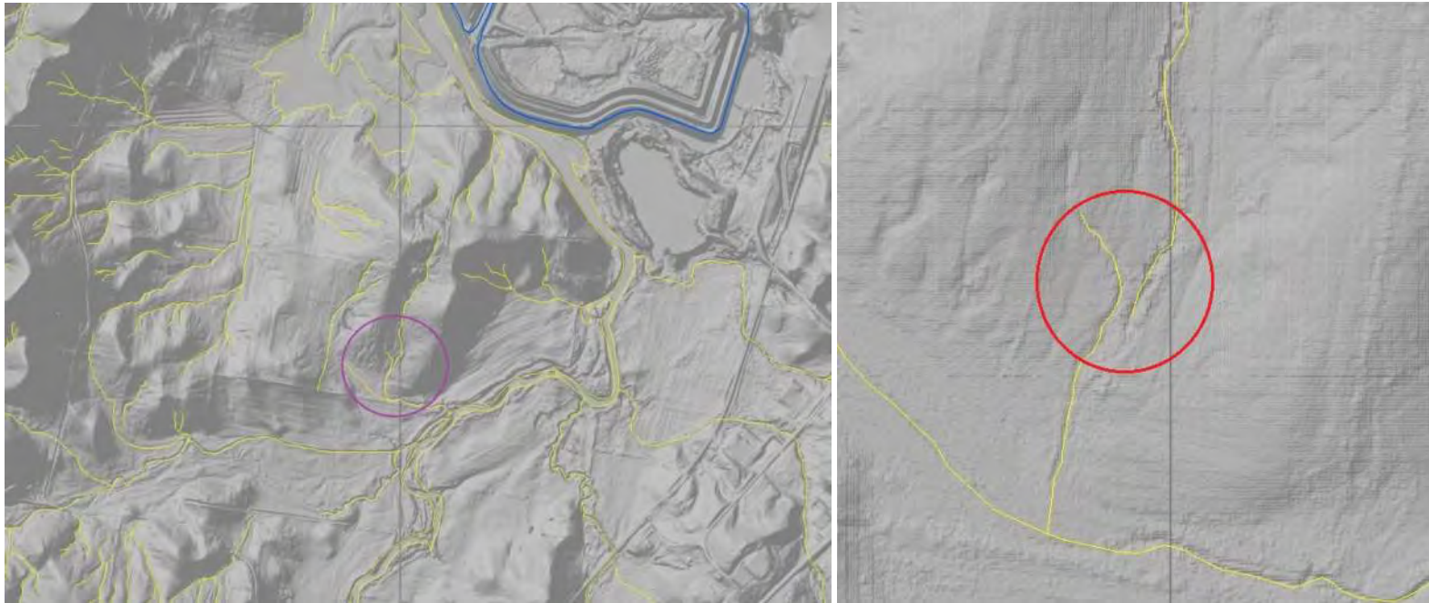
Figure 7. Potential active fault approximately 0.6 miles southwest of the Cumberland Fossil Plant (left). Close-up showing mapped drainage pattern and interpreted off-set (right).
