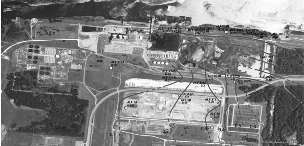
Figure 5 Estimated Drawdown in MRVA Aquifer Monitoring Wells During Memphis Aquifer Pumping Test (values in black, contours in blue; from USGS, 2018)
